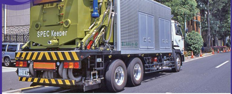
This is a machine that removes material stuck in the gaps of drainage pavements to regain the draining function.
